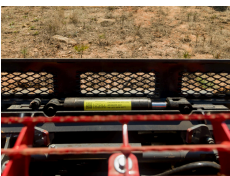
MESH PANELS FOR OPERATOR VISIBILITY
